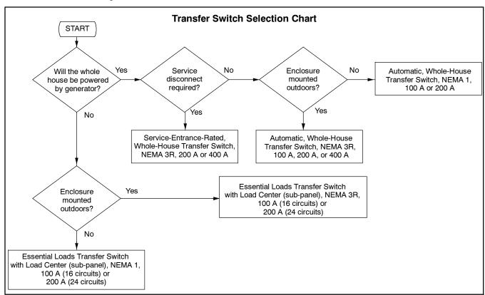
**Note:** RXT transfer switches are compatible with the 14RESA, 20RESA, 38RCL, and 48RCL models only. RDT transfer switches will work with all single-phase 8.5-125 kW generator sets.
